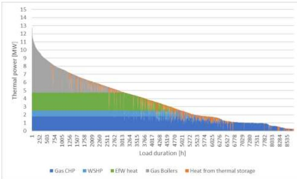
Figure 6-5 Modelled load-duration curve – full Network 3 (Gas CHP, WSHP and EfW)
