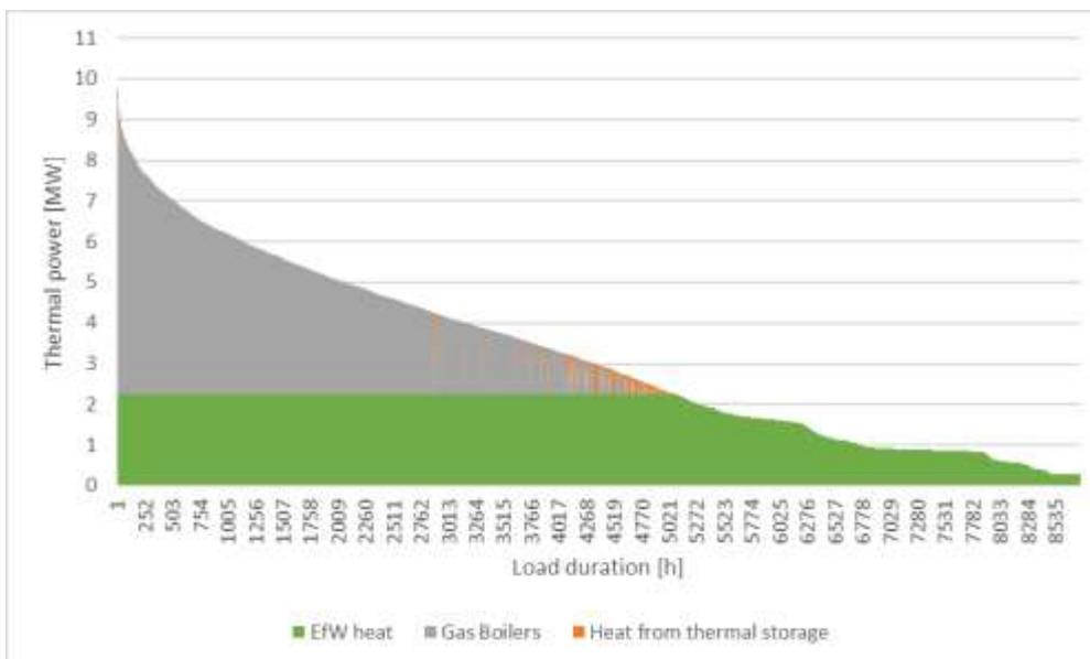
Figure 5-3 Modelled load-duration curve – full Network 2 (EfW)
