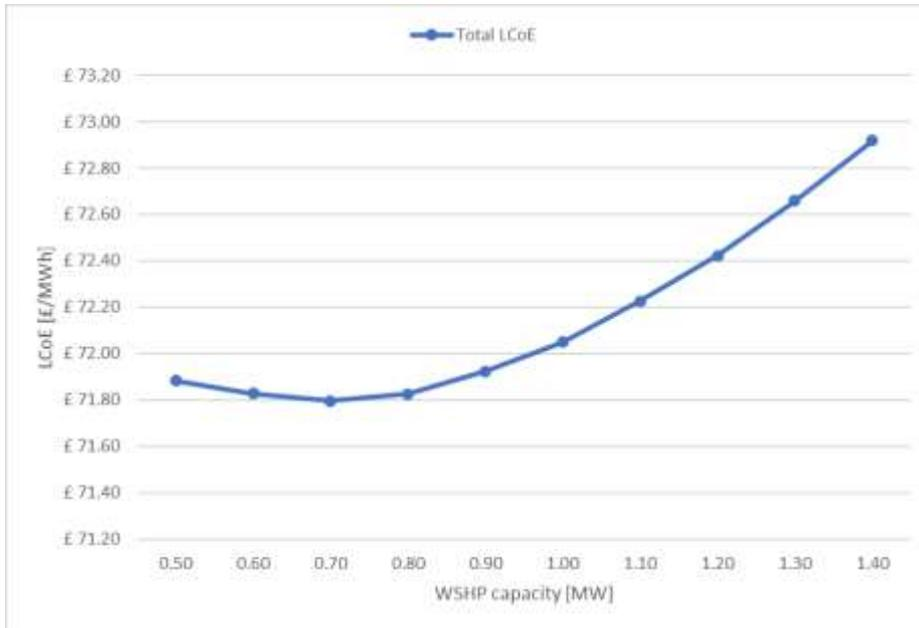
Figure 4-3 Capacity optimisation results - Network 1 (WSHP).
