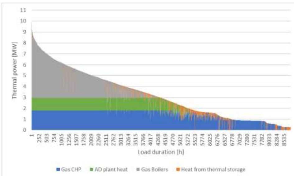
Figure 5-7 Modelled load-duration curve – full Network 2 (Gas CHP and AD plant)
