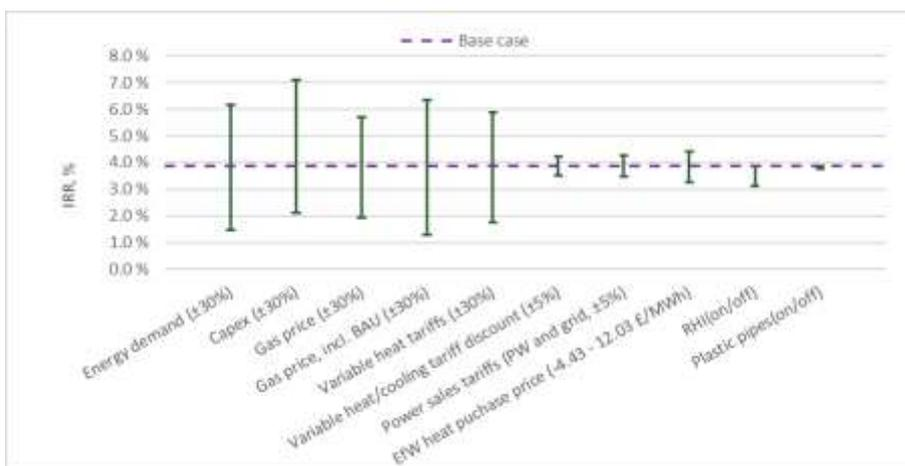
Figure 6-14. IRR sensitivities - Network 3 (Gas CHP & EfW & WSHP)<sup>24</sup>
