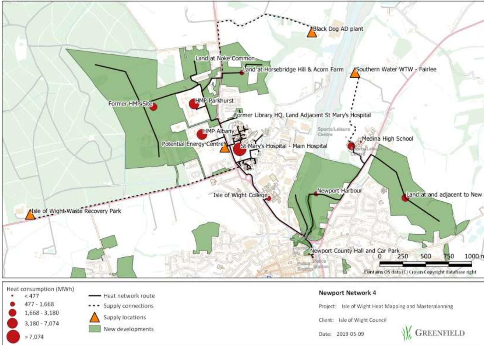
Figure 7-1. Network 4 - heat network and connections.
