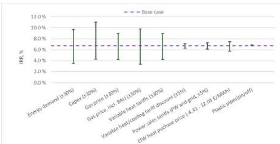
Figure 5-15. IRR sensitivities for Network 2 (Gas CHP & EfW)<sup>17</sup>
