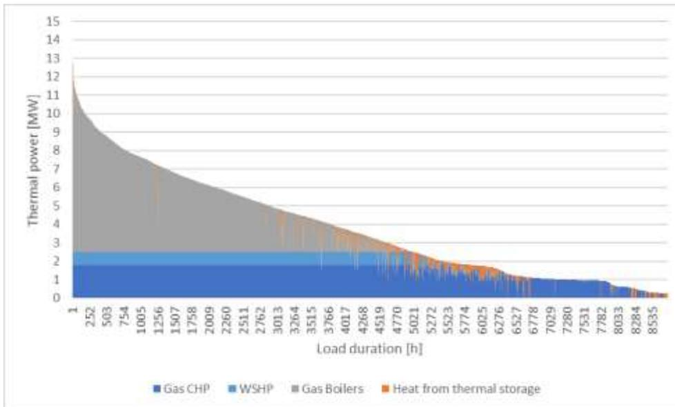
Figure 6-3 Modelled load-duration curve – full Network 3 (Gas CHP and WSHP).
