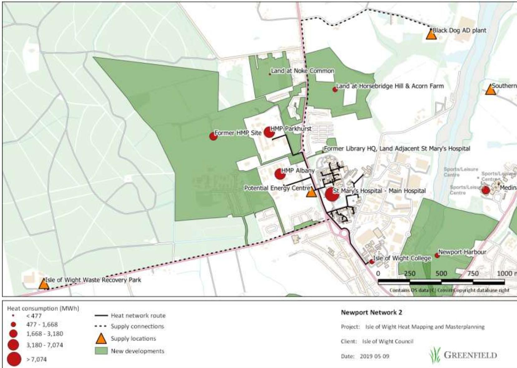
Figure 5-1. Network 2 (Hospital and HMP IoW) - heat network and connections.
