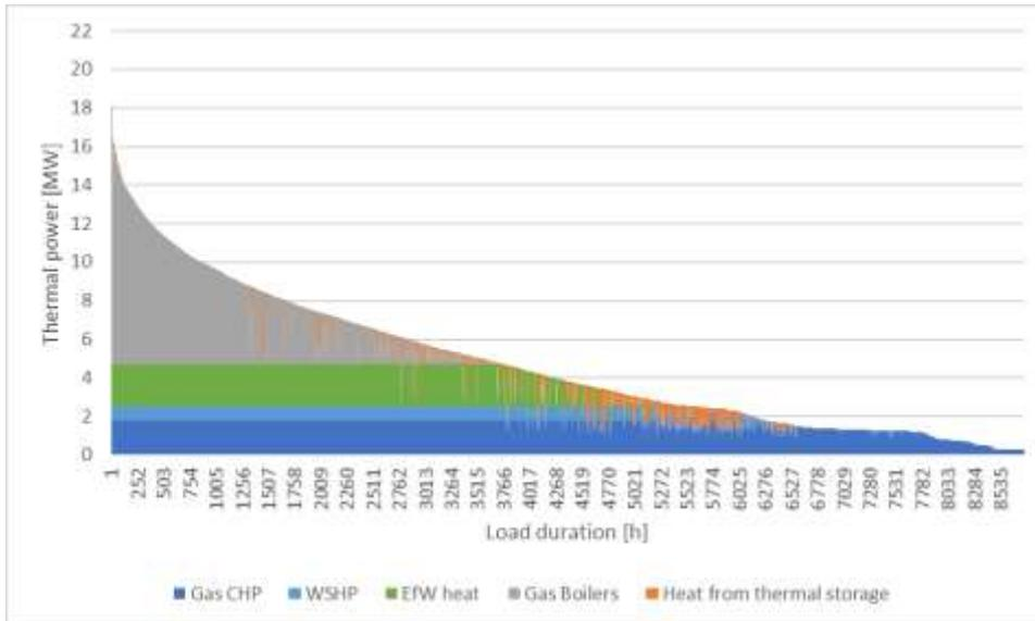
Figure 7-5 Modelled load-duration curve – full Network 4 (Gas CHP, WSHP and EfW)
