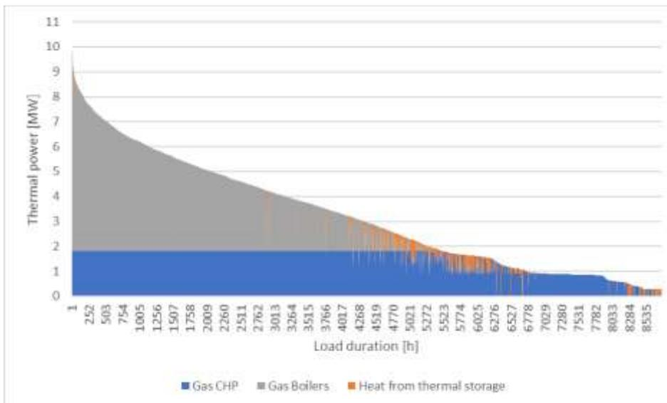
Figure 5-5 Modelled load-duration curve – full Network 2 (Gas CHP).
