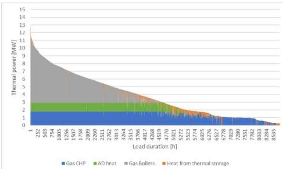
Figure 6-6 Modelled load-duration curve – full Network 3 (Gas CHP and AD heat purchase)
