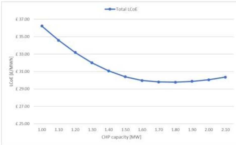
Figure 5-4 Gas CHP capacity optimisation results for Network 2.
