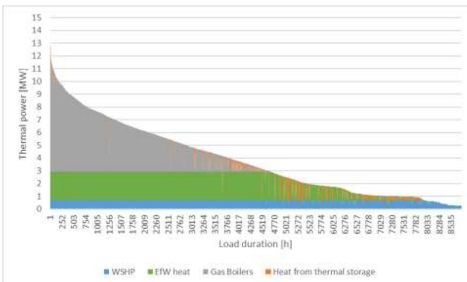
Figure 6-4 Modelled load-duration curve – full Network 3 (WSHP and EfW)
