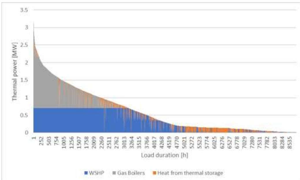
Figure 4-4 Load-duration curve –Network 1 (WSHP).
