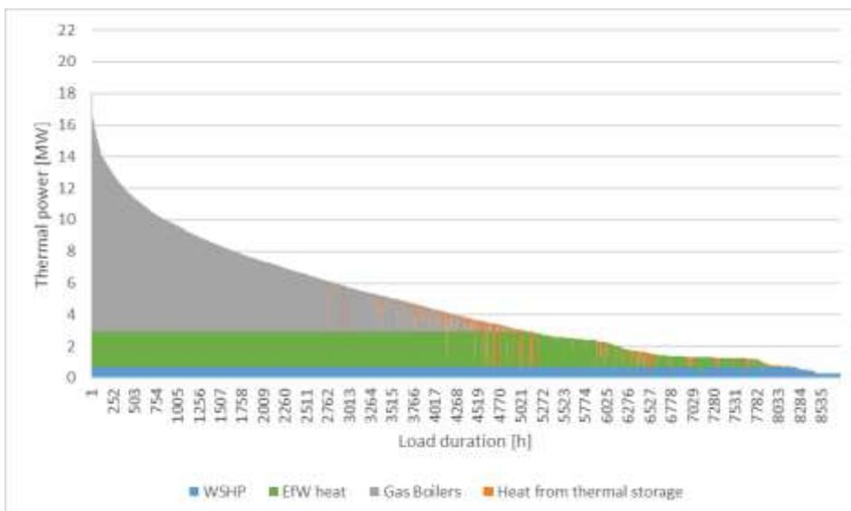
Figure 7-4 Modelled load-duration curve – full Network 4 (WSHP and EfW)
