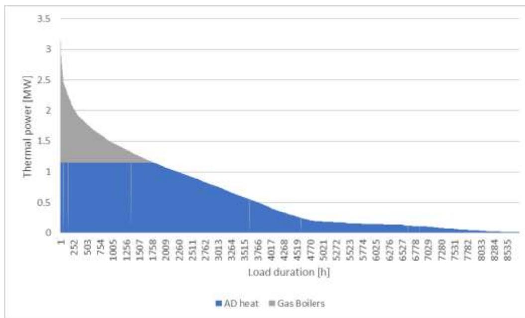
Figure 4-5 Modelled load-duration curve - Network 1 (Black Dog heat recovery).
