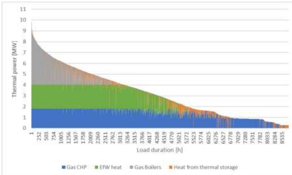
Figure 5-6 Modelled load-duration curve – full Network 2 (Gas CHP and EfW)
