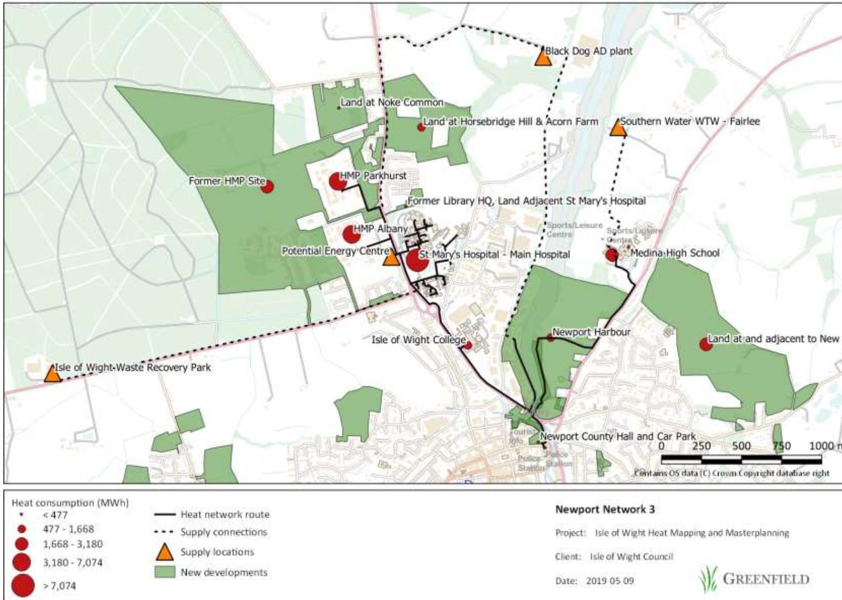
Figure 6-1. Network 3 heat network and connections.
