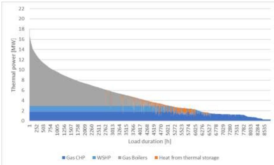
Figure 7-3 Modelled load-duration curve – full Network 4 (Gas CHP and WSHP)
