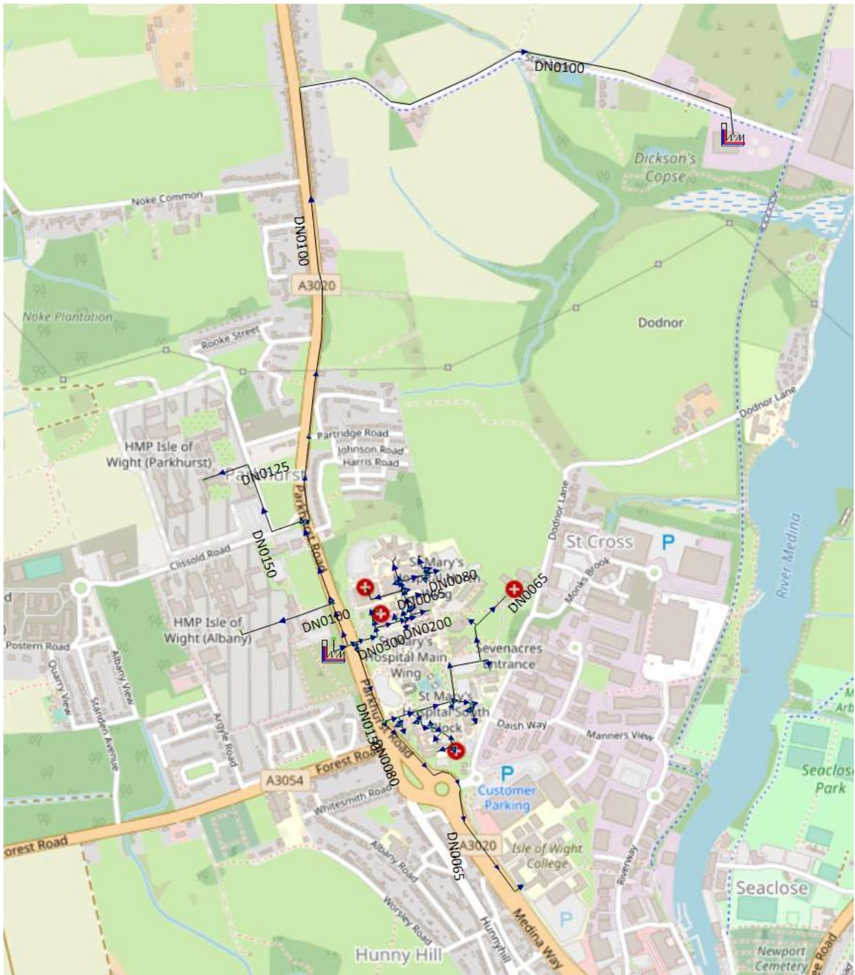
Network 2 Hospital and HMP loW zone (Gas CHP & AD) pipe dimensions.
