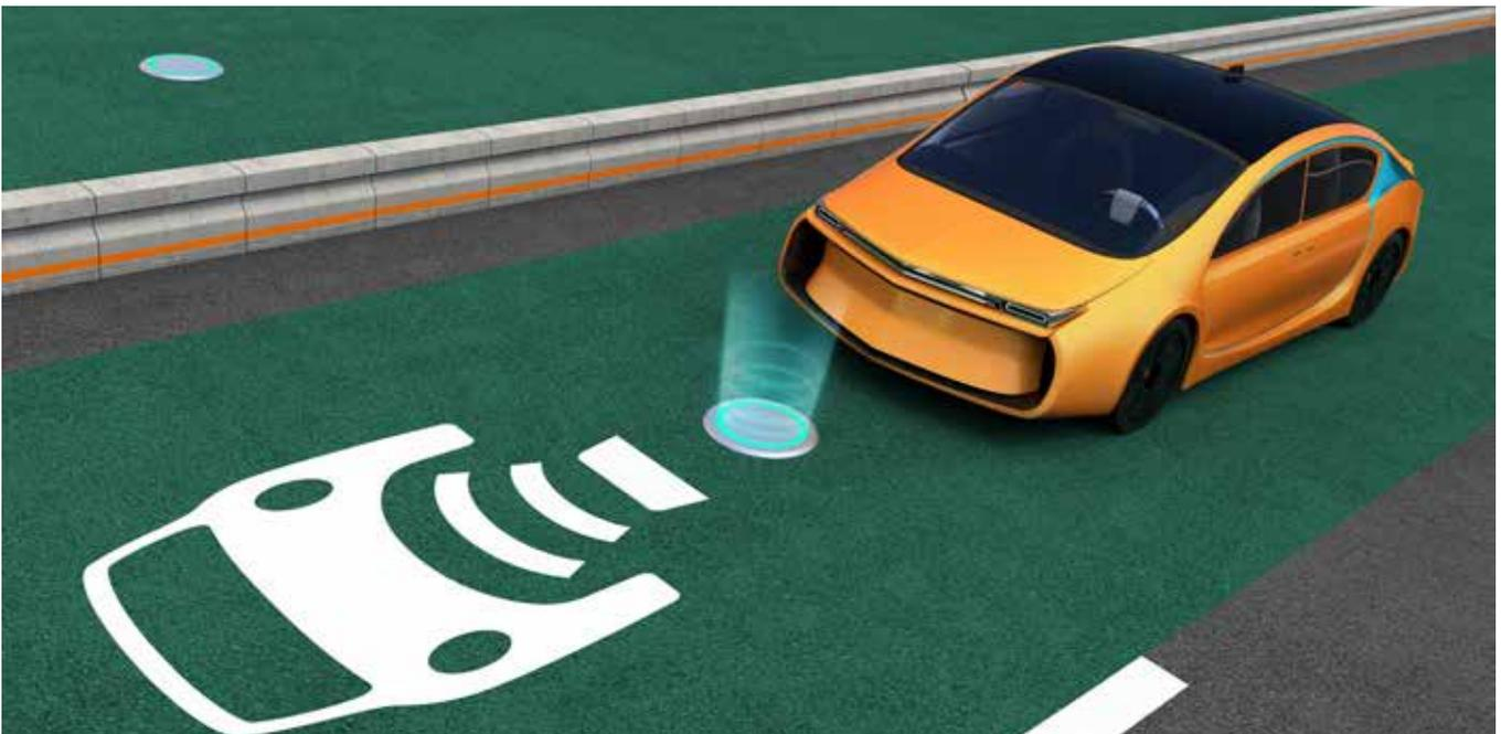
Wireless charging systems are likely to be difficult to install and may have limited applications. Vehicles will have to be manufactured with wireless charging capability and a system for measuring the energy drawn and paying for it will have to be developed. It is, however, a very promising technology for vehicles that are static for short periods, such as taxis, buses and vehicles waiting to board a ferry, and is expected to be commercialised during 2025-2030.
