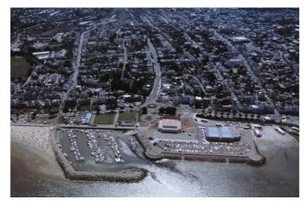
Ryde included sealing off the inlet of Monktonmead stream and construction of houses in the floodplain behind (which have a history of flooding). There is now 7km of continuous defences from Ryde to Seagrove Bay, and a pumping station on the promenade to help manage the flood risk. These defences also form the popular sea front promenade walk from Ryde to Seaview
