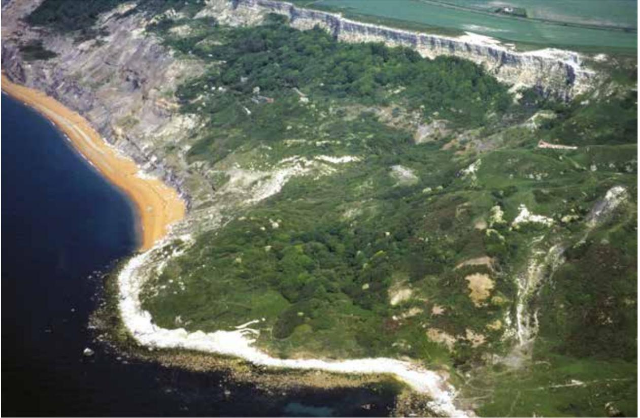
*The massive debris lobe extending into Watershoot Bay near Blackgang following the Gore Cliff rockfall of July 1928. The failure from the rear scarp blocked the old Undercliff Road between Niton and Blackgang and caused collapse of the coastal slope which had become saturated following several months of rainfall.*
