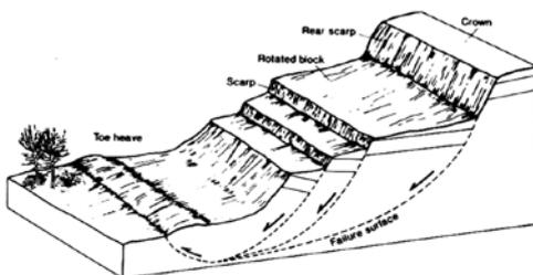
*Multiple-rotational slides (left) involving a series of slipped, back-tilted blocks each underlain by a circular failure surface that merge to form a common basal shear surface. These mainly occur at the rear of the Undercliff*
