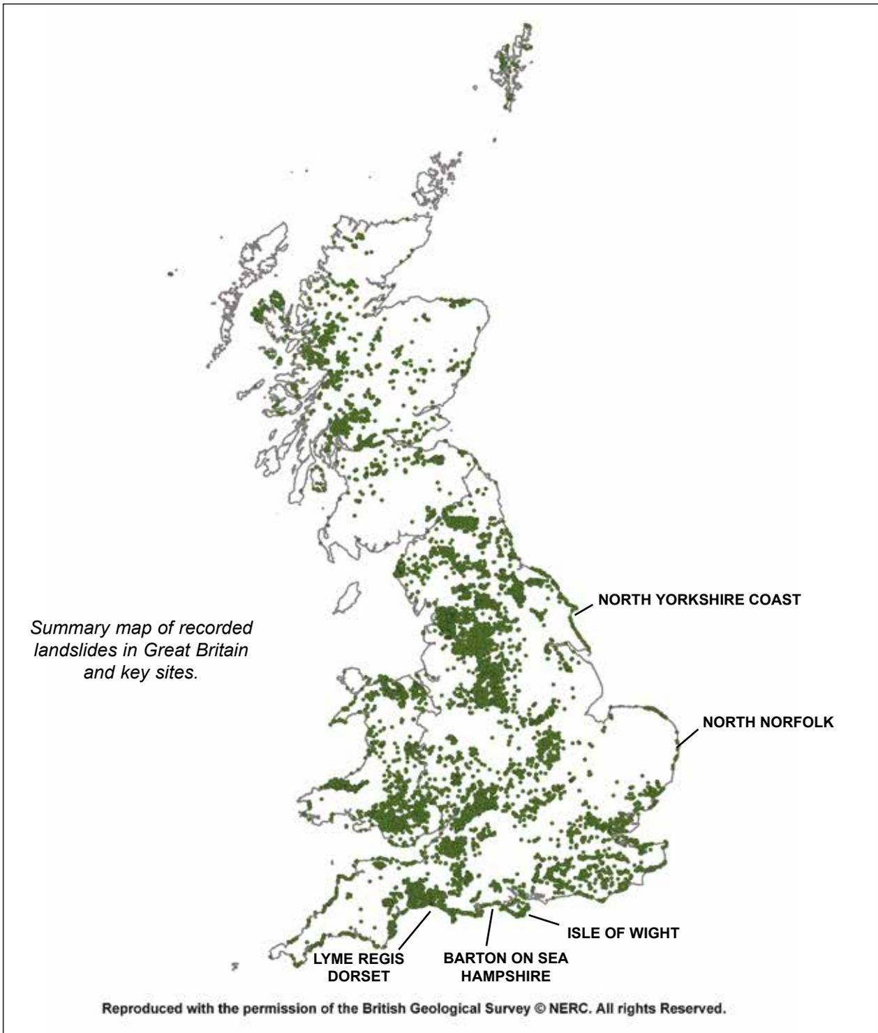
Location of landslides recorded in the British Geological Survey's National Landslide Database. The National Landslide Database is being developed as the definitive source of information on landslides in Britain . It currently holds 14,200 records of landslides, and new records are being added every year.
