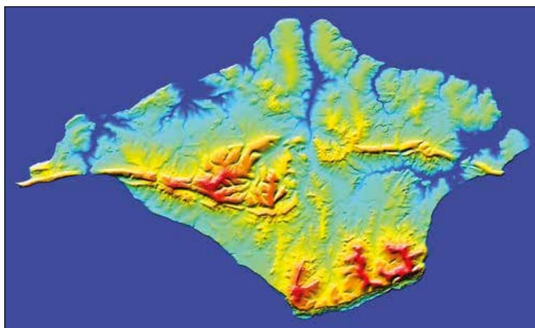
*A computer-generated image of the Isle of Wight. The yellow and red colours represent the high downland of the island. The tract of slipped land on the south coast, the Undercliff, may be seen at the bottom of the image. (Halcrow, 2006)*
