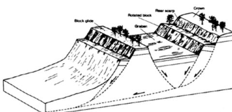
*Compound slides (left) characterised by markedly non-circular shear surfaces. This type of slide involves the lateral displacement of a block forming an elongate ridge and the creation of a low-lying depression or graben immediately upslope, for example at Newport Road, Upper Ventnor and at Park Avenue, Ventnor*
