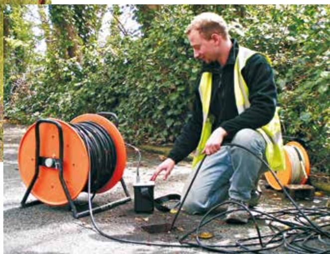
Taking inclinometer readings from a borehole along the Undercliff.
