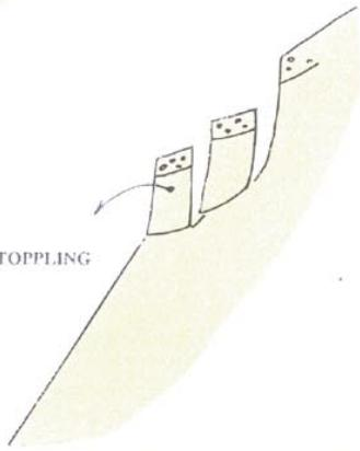
CIRCULAR FAILURE FOLLOWED BY TOPPLING FAILURE INVOLVING RELATIVELY LIMITED GROUND MOVEMENT
