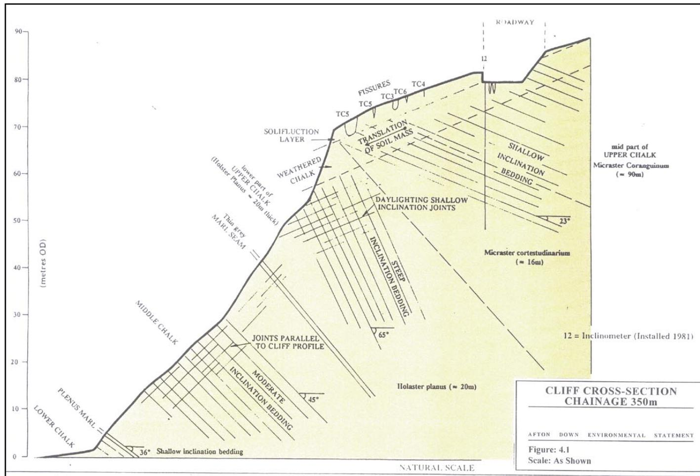
Figure G10.4 Cross section through the Afton Down cliff.
