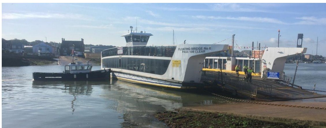
Figure 5. Use of push boat against FB6 (Source: Isle of Wight Council)
