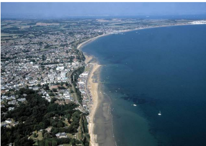
Left: View north-west from Shanklin across Sandown Bay, towards Culver Cliff (Chalk headland) in the distance. The former sea cliffs are stabilised in the centre of the bay and sediment transport is from south to north-west, forming important amenity beaches (Isle of Wight Council).
