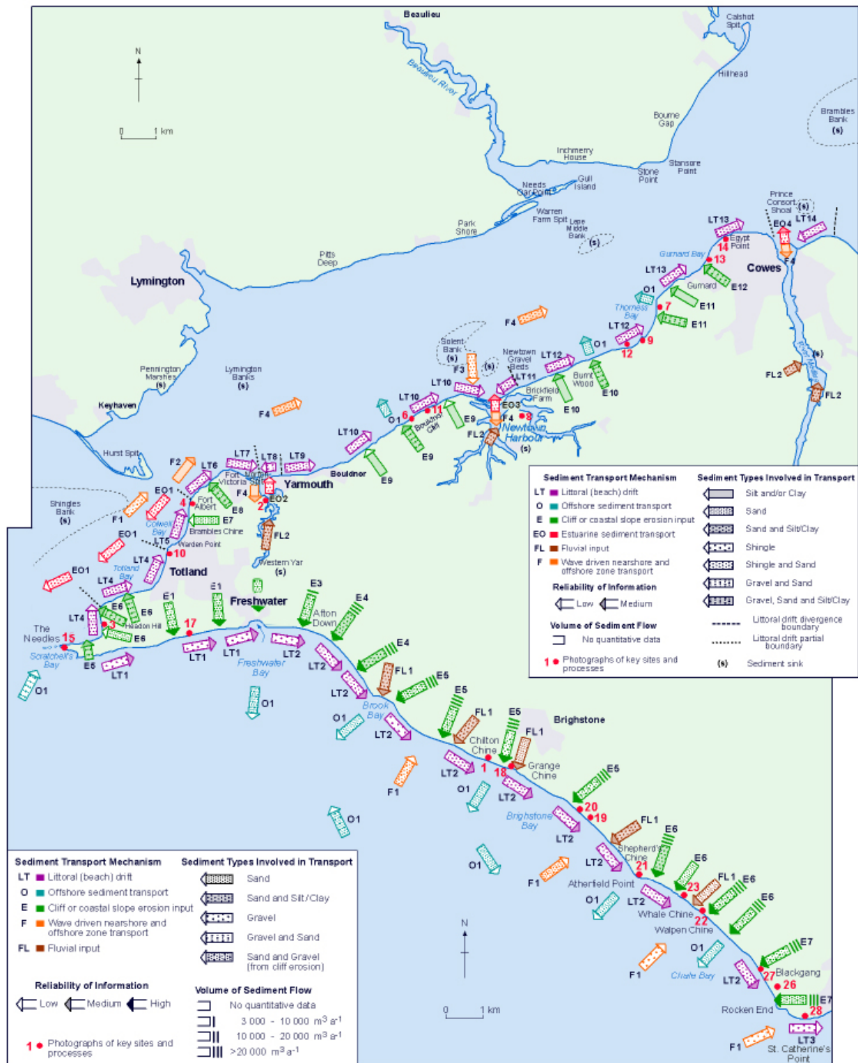
Sediment transport sources, pathways and sinks on the west coast, from SCOPAC Sediment Transport Study, 2004.
